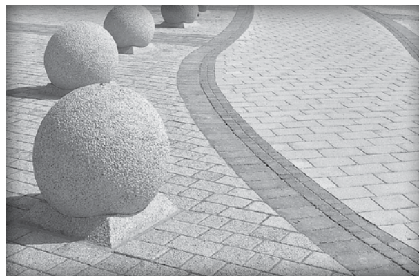
Figure 4. Light colored paving units reflect light and help reduce micro-climatic temperatures.
